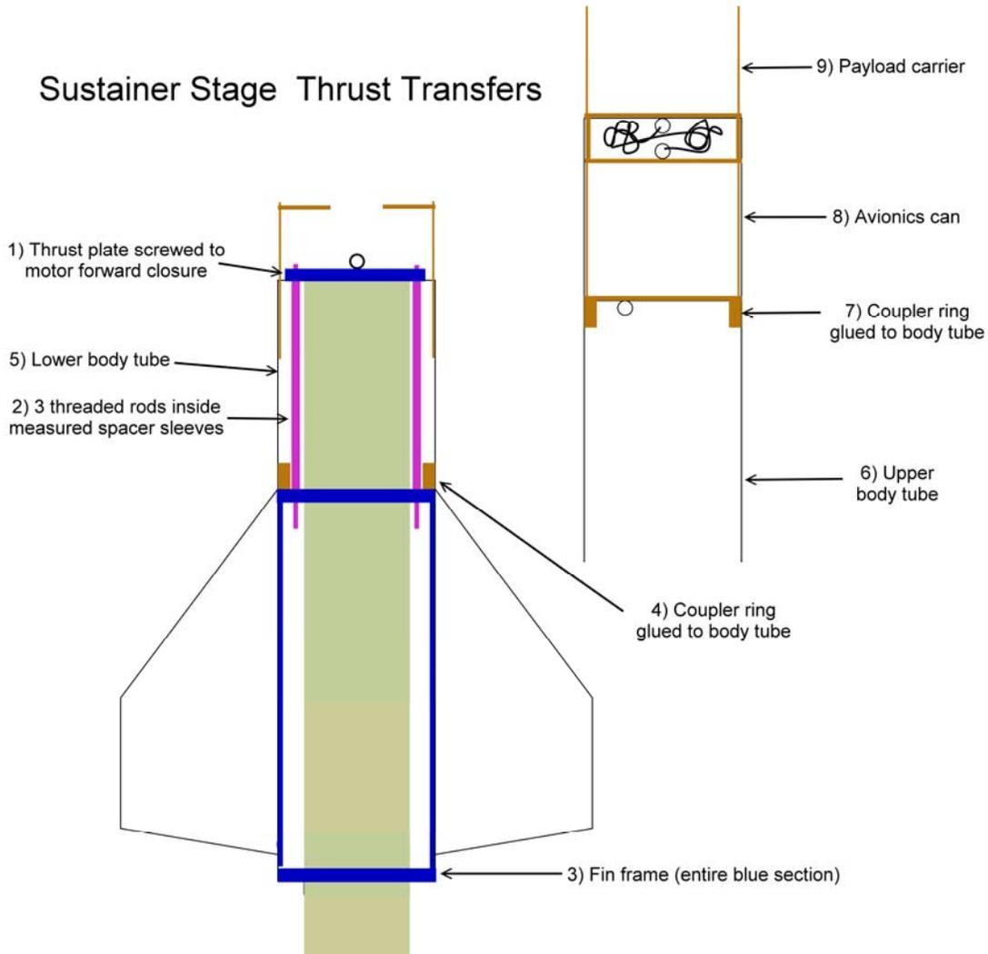
**Figure 8. Sustainer Thrust Transfer Path**
