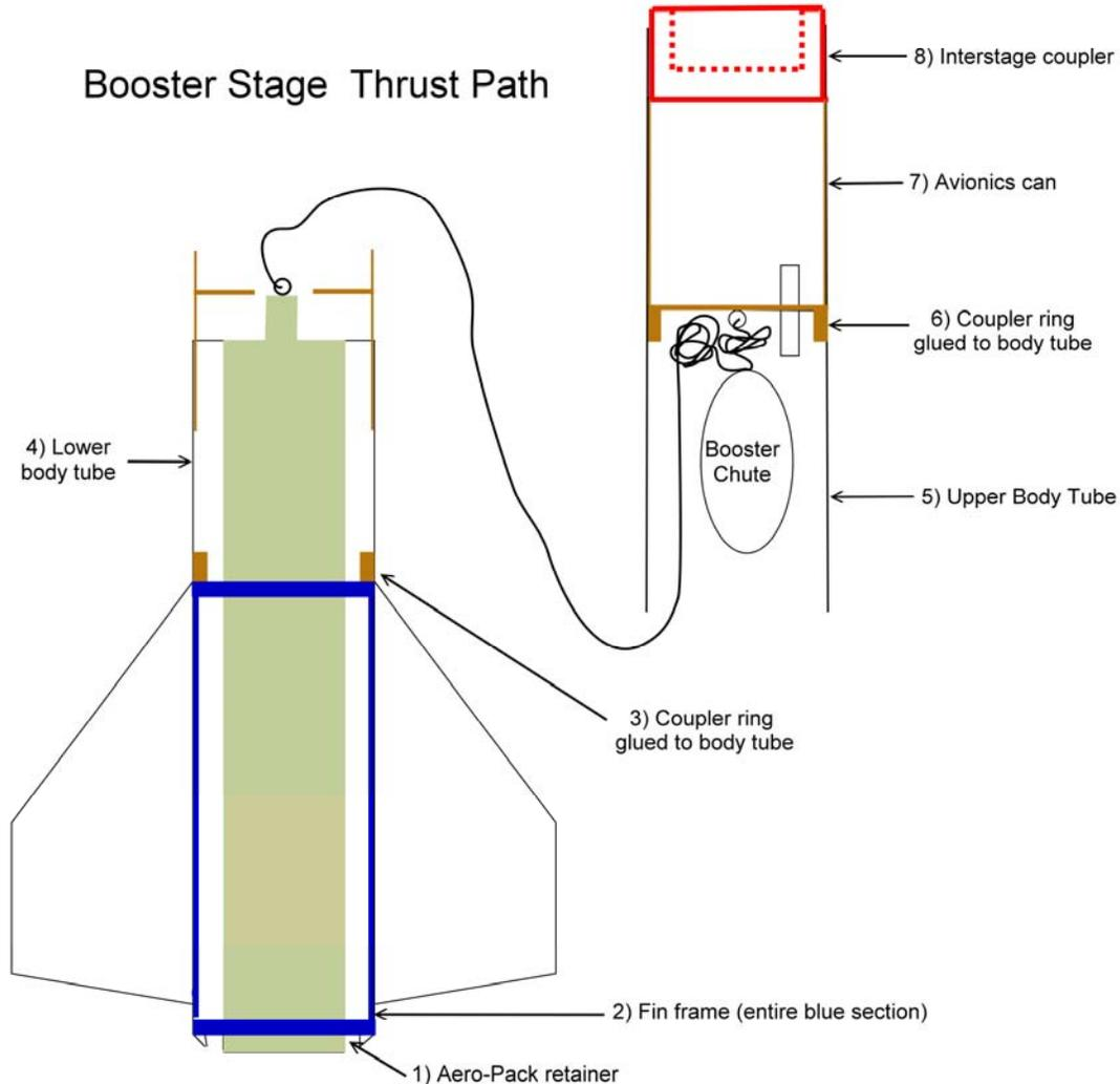
**Figure 6. Booster Thrust Path**
