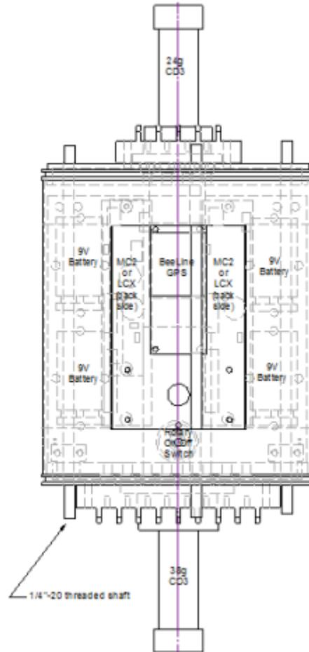
The computers are programmed to ignite an electric match at apogee to trigger a CD3 CO<sub>2</sub> ejection unit and deploy the main parachutes. Six seconds after apogee a second electric match is ignited, which fires a black powder charge to separate the nosecone from the upper airframe and deploy the payload. The CD3 has provisions for two electric matches. One is wired to the MC2 the other is wired to the LCX.
