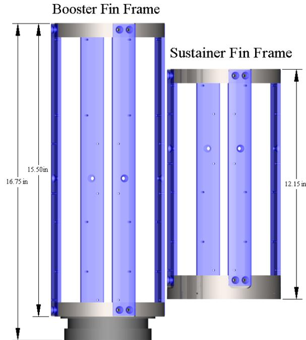
**Figure 4. Fin Frames (Booster shown with motor retainer)**
